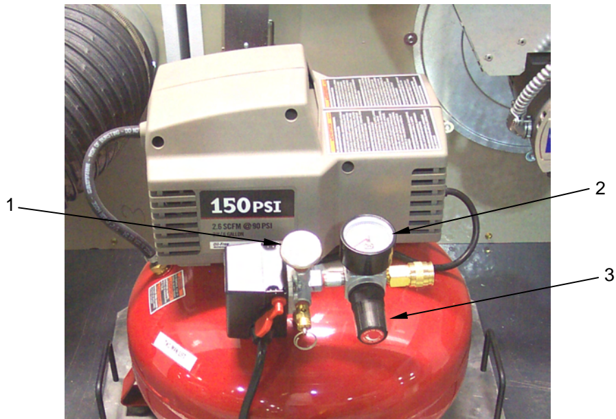
Figure 12. Verify Air Compressor Regulator Pressure Reads Zero.
