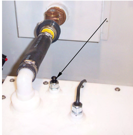
Figure 14. Lifting the Manual Override on Waste Tank.
