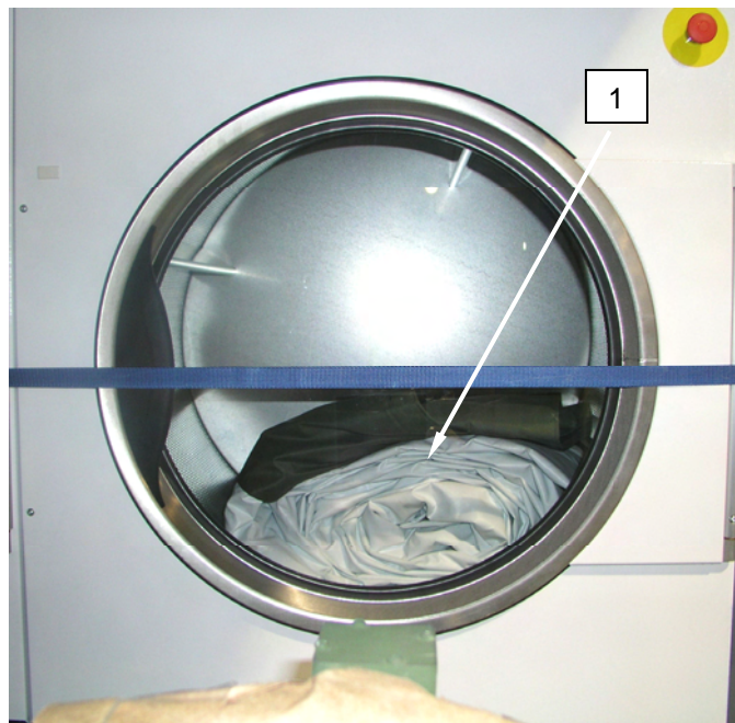
Figure 11. Removing Laundry Boot Wall from Dryers.
