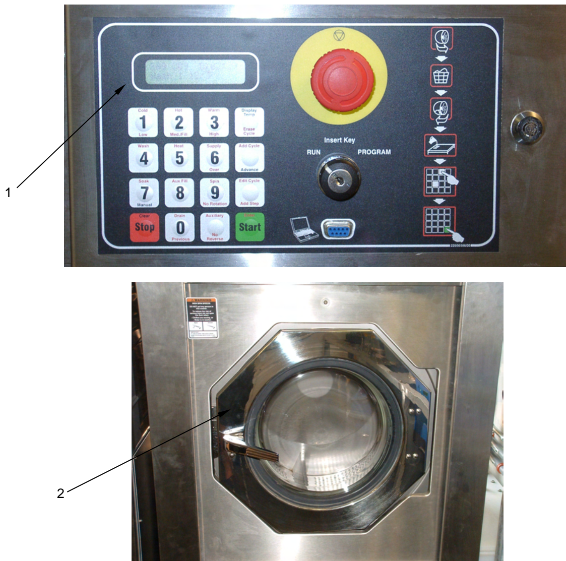
Figure 1. "Door" Error on Washer Display.
