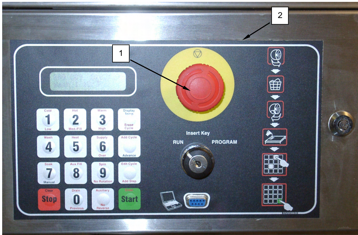
Figure 3. Replace the Microprocessor Display Overlay.
