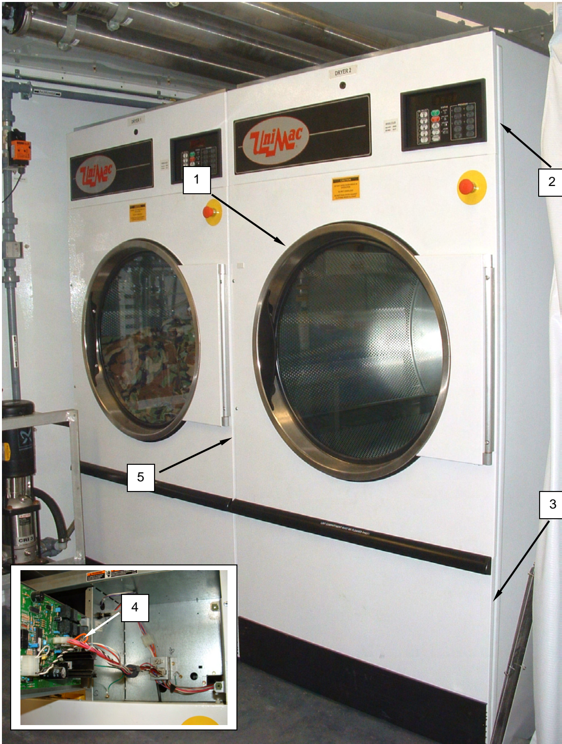
Figure 3. Replace the Dryer Emergency Stop Switch.
