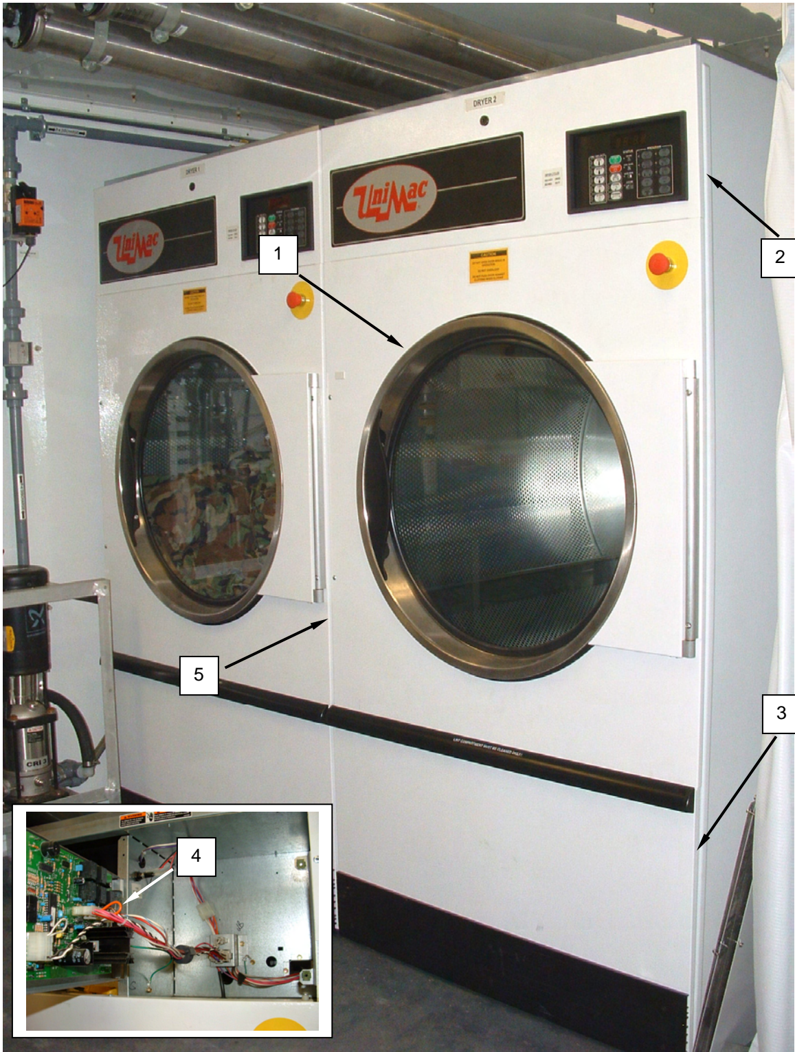
Figure 1. Test the Dryer Emergency Stop Switch.
