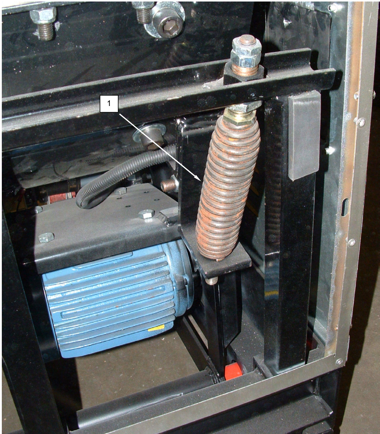
Figure 2. Inspect the Washer Springs.
