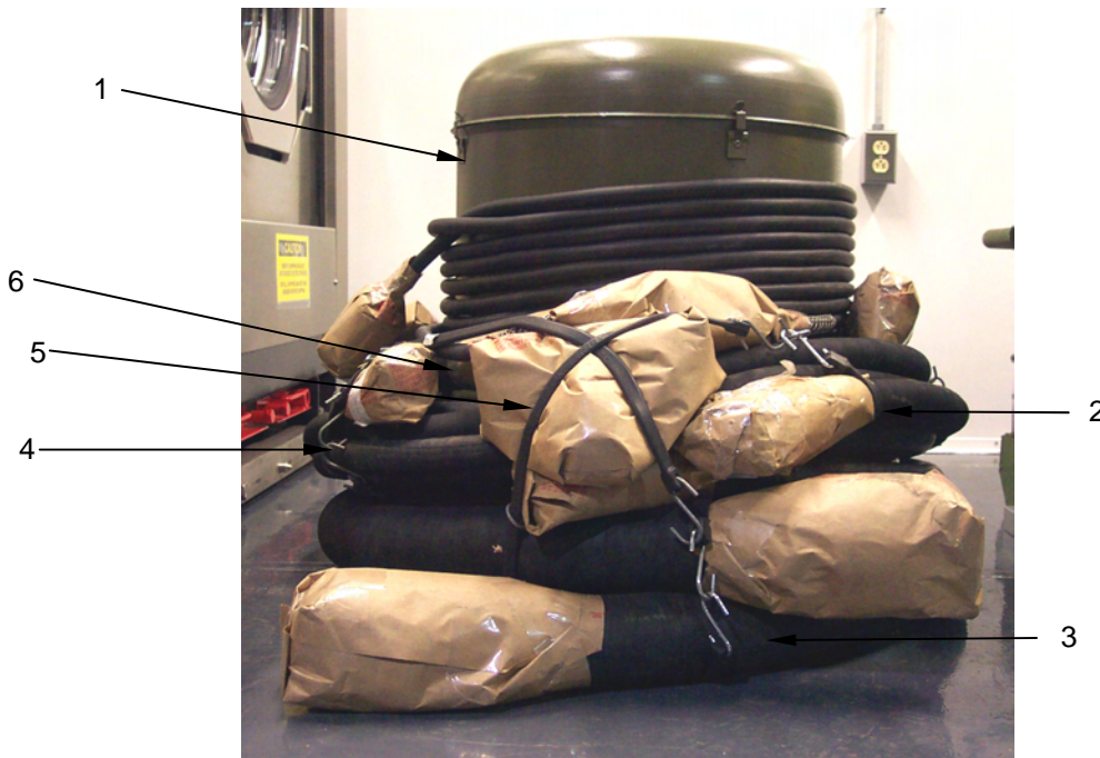
Figure 3. Packing Exhaust Fan Components and Hoses.
